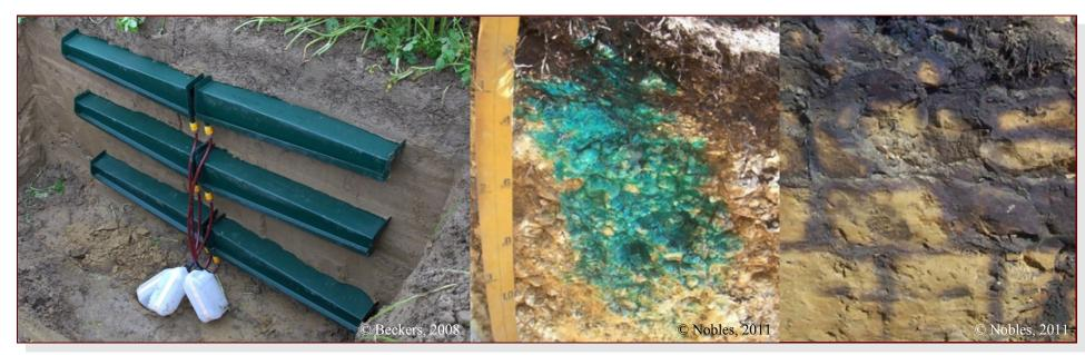
Figure 6 Dye tracing experimentation
