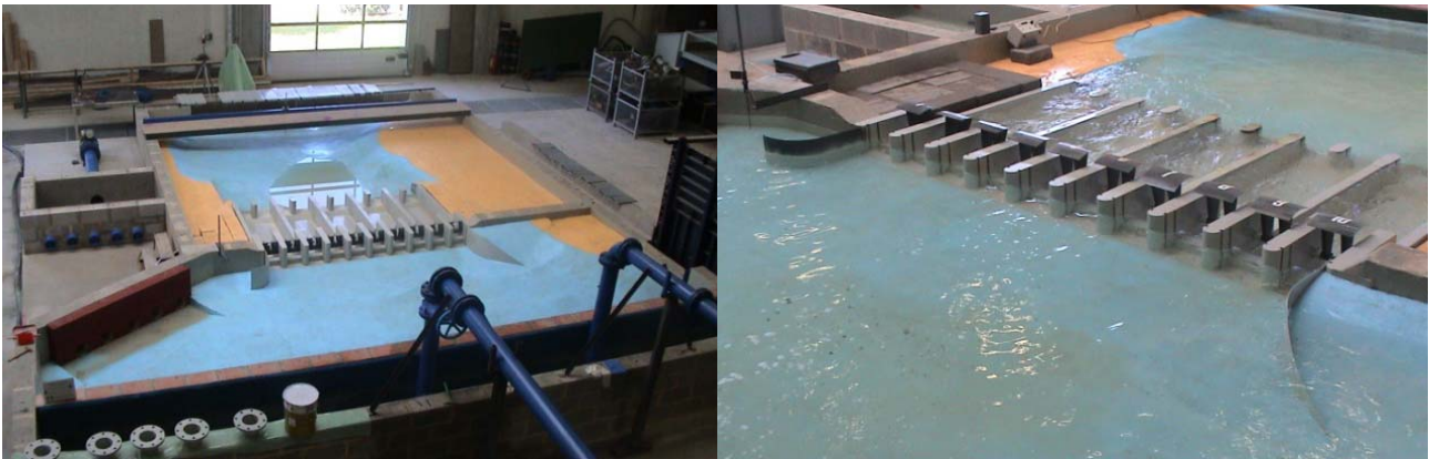
Fig. 4 - General view of the scale model (left) and details of the gated weir and stilling basin (right)
