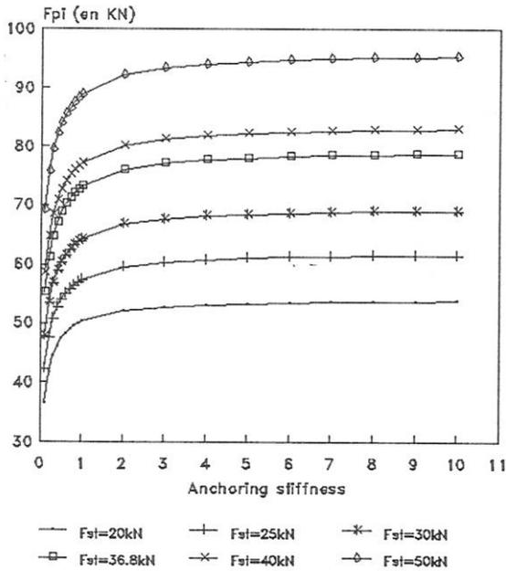
Figure 6: Fpi versus anchoring stiffness results
