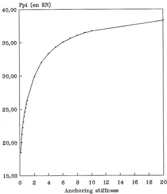
Figure 3: Fpi versus anchoring stiffness results
