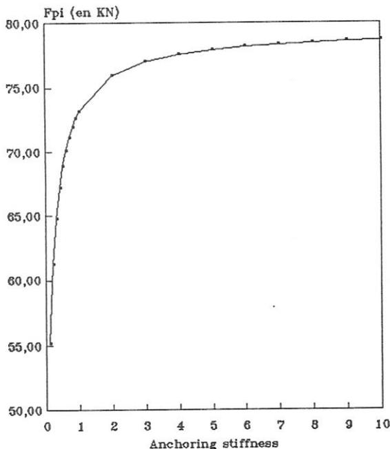
Figure 4: Fpi versus anchoring stiffness results
