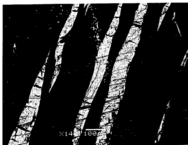
FIGURE 2. Triphylite (dark grey) including lamellae of sarcopside (white), Cañada pegmatite, Spain (sample SS-3, BSE image).
