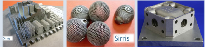
SLM smart structures made by Sirris (TipTopLam and Compolight projects)
