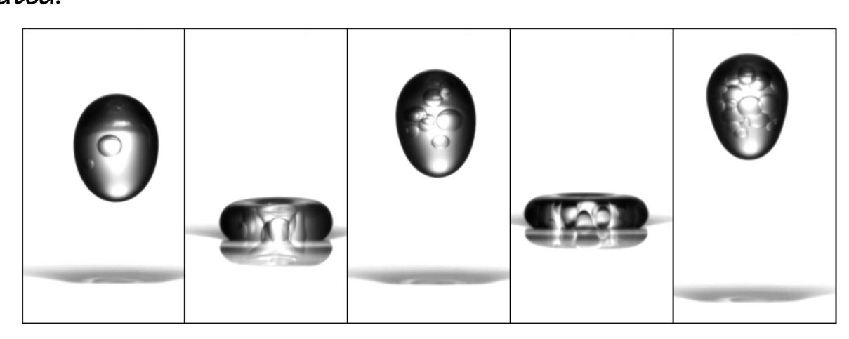
When the forcing acceleration is higher than a certain threshold, compound drops can bounce on the surface. We show that above another acceleration threshold some oil contained in the shell enters in the inner water droplet forming a stable double emulsion.
