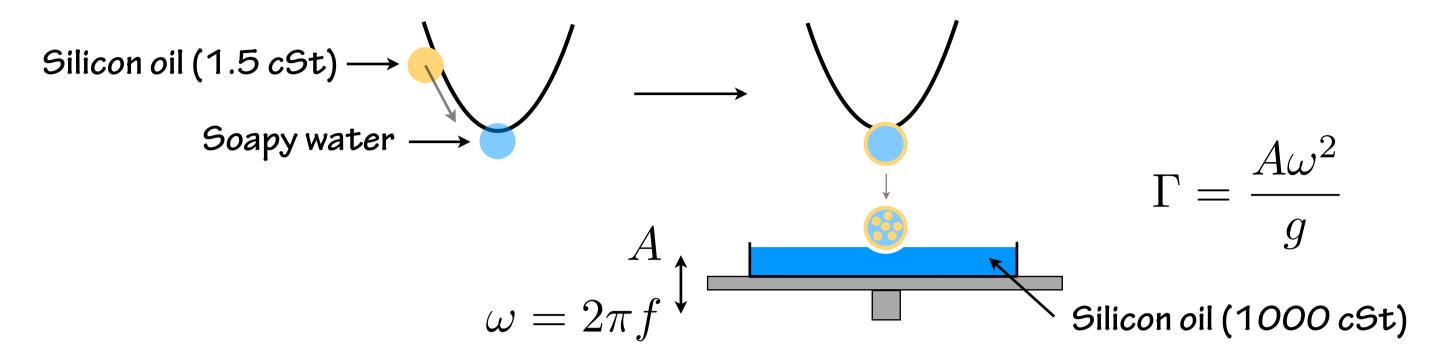
When the forcing acceleration  $\Gamma$  is higher than the bouncing acceleration threshold  $\Gamma_{\text{th}}$ , the compound drop bounces on the surface. Above another threshold,  $\Gamma_{e}$ , an emulsion is initiated in the compound drop.
