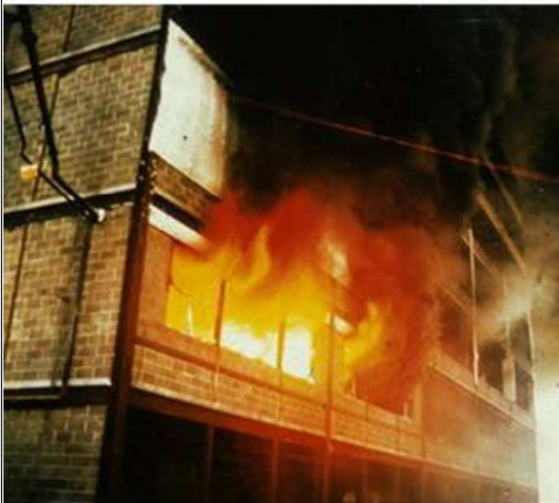
2 nd corner test: fire load (above) and during the test
