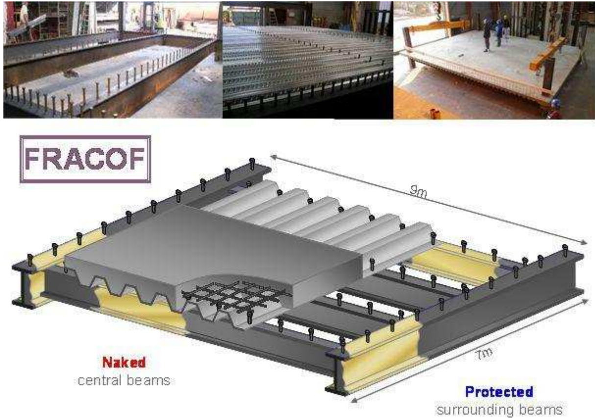
Fig. 3: Layout of the specimen tested in the Fracof project
