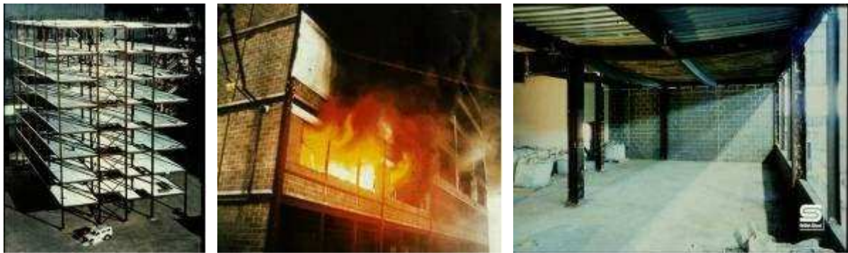
Fig. 1. Cardington test building and one of the fire tests
