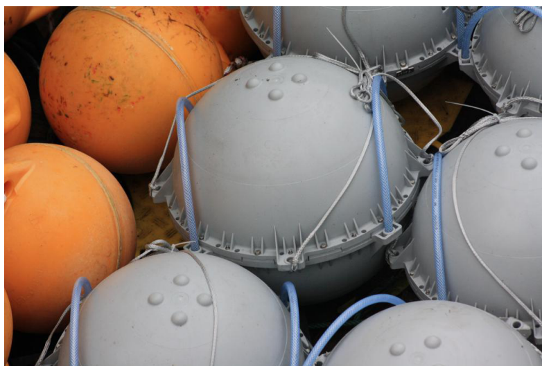
Figure 4.11: The radio-wave emitting parts of the Argos drifting buoys are located in the gray spheres. A drogue (not shown here) was attached to each of them in order to follow the current.
