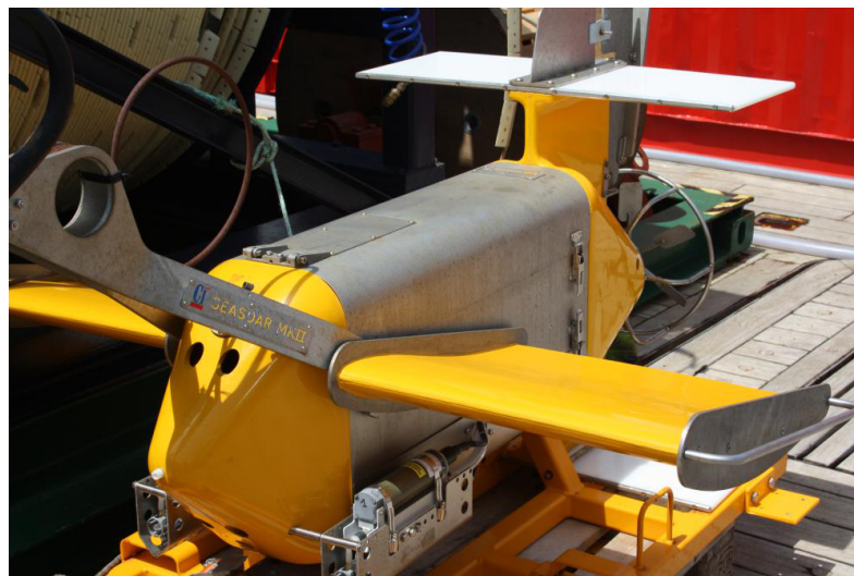
Figure 4.6: The SeaSoar Mk II vehicle employed for the measurements has the following characteristics: length: 2 m; height: 0.98 m; width: 1.60 m, weight: 150 kg; maximal speed: 12 kn (22 km/h). Technical document available at http://www.chelsea.co.uk/Factsheets/SeaSoar04.pdf
