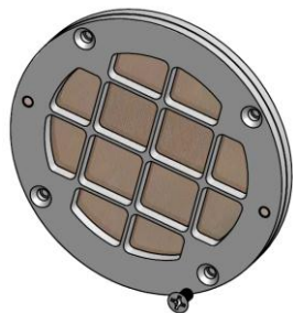
Fig. 8: Frame filter concept, clamping the meshed foil filter. Courtesy: LUXEL.
