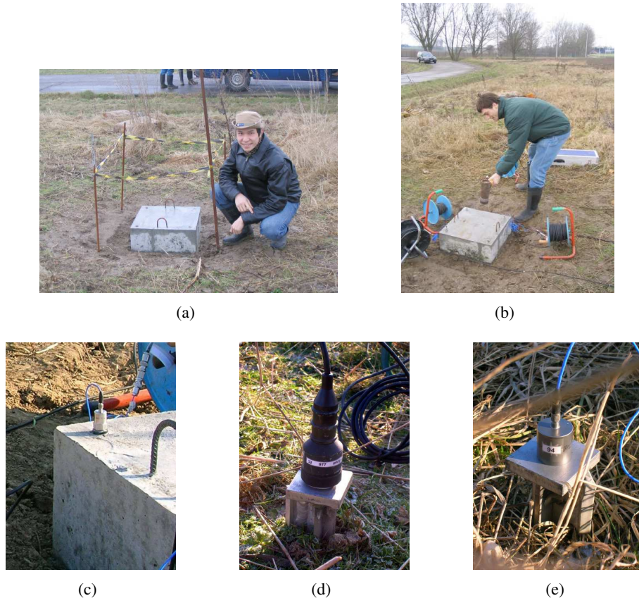
Figure E.3: Site of Lincent: (a) concrete foundation, (b) instrumented hammer, (c) accelerometer mounted on the foundation and (d, e) accelerometers in the free field.
