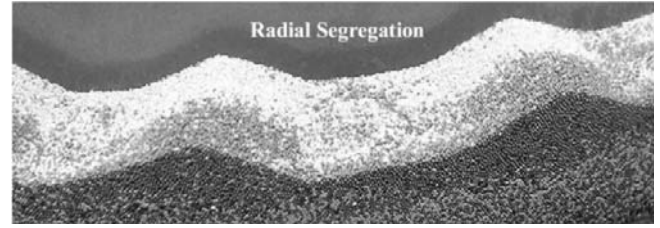
Fig. 9. Radial segregation is characterised by large grains preferentially situated close to the outer wall while the small ones go near the inner wall. Mixture M1 in Setup 2. frequency f = 1 \text{ Hz} and amplitude A_2 \text{ cm} .
