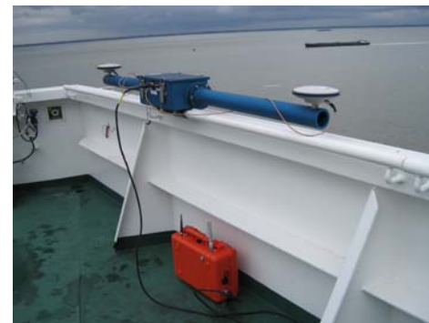
Figure 10. Vessel monitoring equipment of Flanders Hydraulics Research for tracking ships during approaches and maneuvers (photo Flanders Hydraulics Research).
