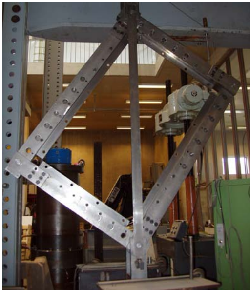
Figure 5 – Global view of the frame for shear tests
