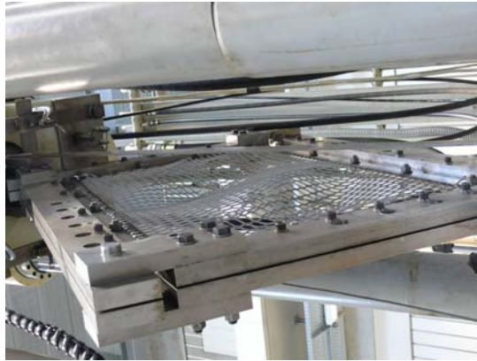
Figure 7 – Buckling shape after testing of specimens
