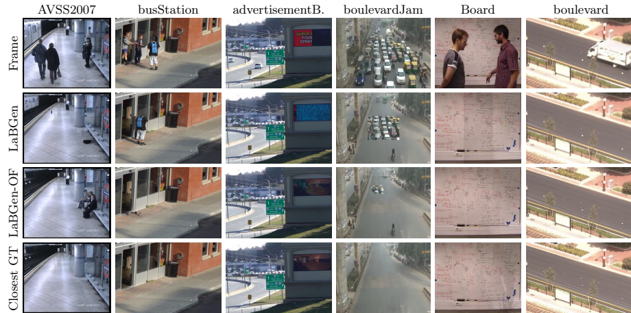
Fig. 5. Background generated for some SBMnet sequences provided with ground-truth (the 1 st row contains a randomly selected frame) by LaBGen [9] (2 nd row), and by LaBGen-OF with its default set of parameters given in Eq. 6 (3 rd row). The 4 th row contains the closest ground-truths to the results of LaBGen-OF. Only sequences where a difference is visually noticeable are shown.
